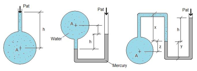
Here, to find A point pressure, pressures are calculated along the tube as +/-. Walls of the tube is exposed to atmospheric pressure, the atmospheric pressure ignored. Let's write the formula for third picture.
