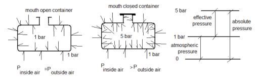
**Example**: How much force act the cover in 20 cm diameter when the inside absolute pressure raised to 1.3 bar in a pressure cooker.
