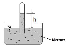
Example: The density of mercury is 13560 kg/m<sup>3</sup> at 15 °C and ambient atmospheric pressure is 1 bar then how much we read the height of the mercury in mm.
